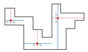
Given an x-monotone rectilinear polygon, write a program to compute the minimum number of sensor units required to completely monitor the polygon.
